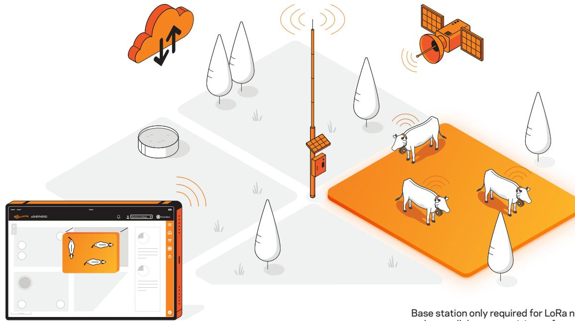
Base station only required for LoRa neckbands - where cellular connectivity on farm is limited.
